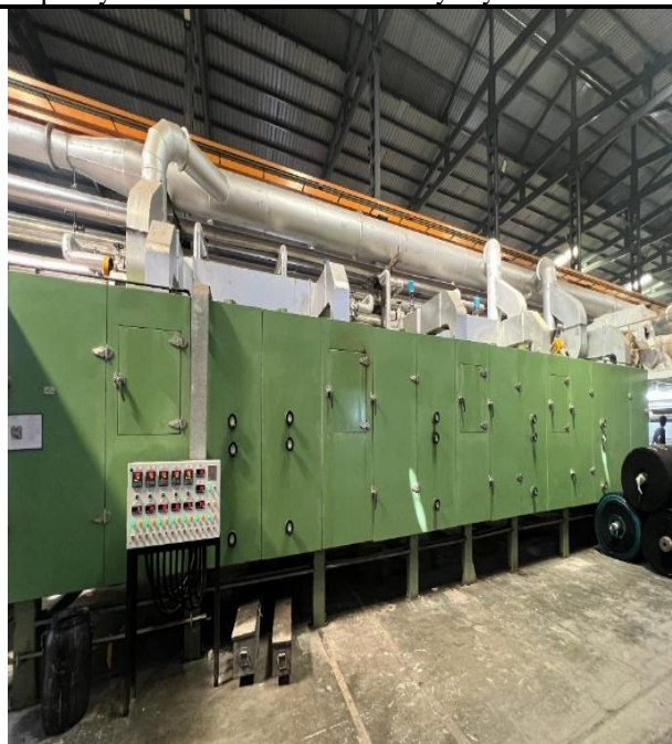
Machinery Name: 15M Oven Location In Plant: Main Plant Use: To make PVC slurry foam to expected thickness or to make PU or PVC slurry dry
