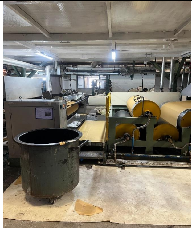
Machinery Name: Adhesive Head Location In Plant: Main Plant Use: Use water to cool down leather & paper temperatures
