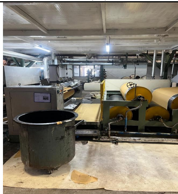
Machinery Name: Adhesive Head Location In Plant: Main Plant Use: Use water to cool down leather & paper temperatures
