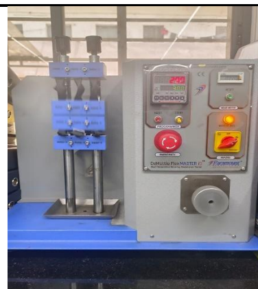
Machinery name: DeMattia Flex Machine Location in plant: Quality Assurance Laboratory Use: To measure the flex Cracking Resistance
