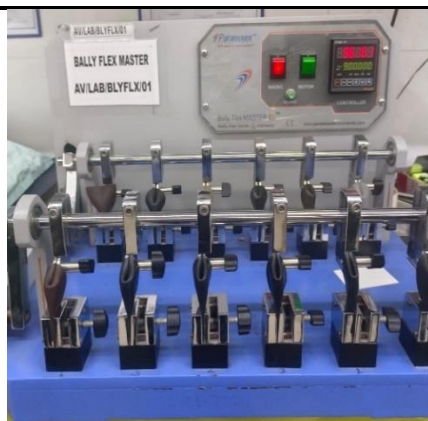
Machinery Name: Bally Flexing Machine Location in Plant: Quality Assurance Laboratory Use: Assesses the flex resistance
