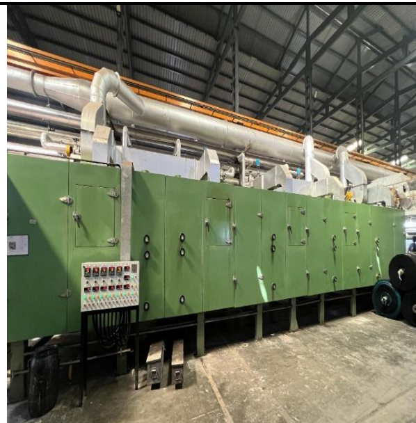
Machinery Name: 15M Oven Location In Plant: Main Plant Use: To make PVC slurry foam to expected thickness or to make PU or PVC slurry dry
