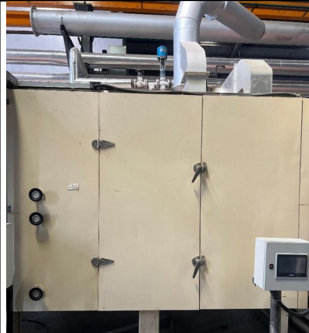
Machinery Name: 3MOven Location In Plant: Main Plant Capacity: To make PU or PVC slurry dry
