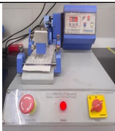
Machinery Name: Croco Meter Location In Plant: Quality Assurance Laboratory Use: To check the color fastness
