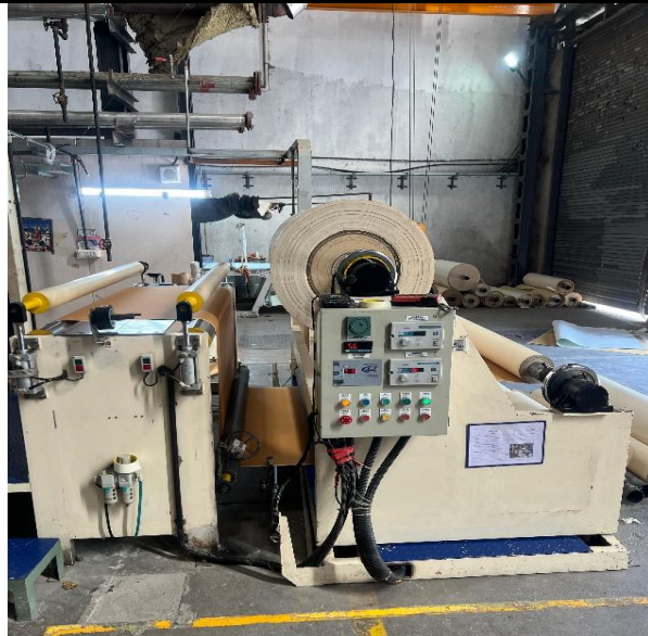
Machinery Name: Unwinder Location In Plant: Main Plant Use: Unwinding Release paper
