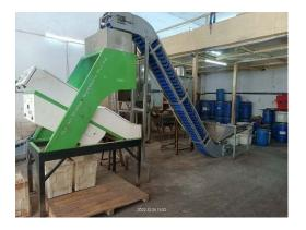
After Peeling, All Kernels (Whether Whole or Broken) are being processed thru Colour Sorter to remove Rejection / Oily Kernel / Dotted Cashew Kernels / Kernels with Minimum Husk and to separate clean Kernels.
