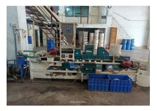
After sorting and Drying, Kernels have been processed thru Nano pix grading Machine. In this process, We are able to separate Kernels into Different Grades with the help of Hitech Camara used in this machine.
