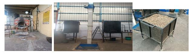
Once Raw Cashew Nuts are dust cleaned, it's getting load thru Elevator in Tank for steaming thru IBR. The process of steam boiling helps in soften the outer shell and removal of this shell with minimal effort. On completion of Boiling all nuts been offloaded in trolley and leave for cooling period.
