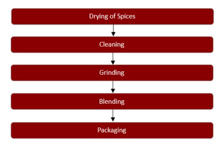
**Drying of spices:** The process begins with the drying of raw whole spices to reduce their moisture content to optimal levels. This step is crucial for preserving the natural oils, flavour, and aroma of the spices while also preventing fungal or microbial contamination. Drying is performed using hot air dryers or solar dryers in a controlled environment, ensuring that the spices are properly conditioned for further processing.
