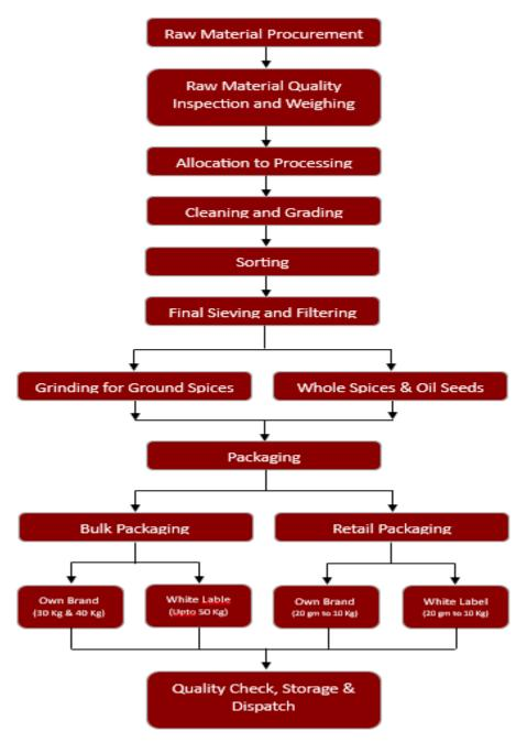
The manufacturing process involves cleaning, drying, sorting, grading, sieving and packing of ground nuts and grain (wheat) such as ground spices like chilli, turmeric, coriander, coriander cumin etc.
