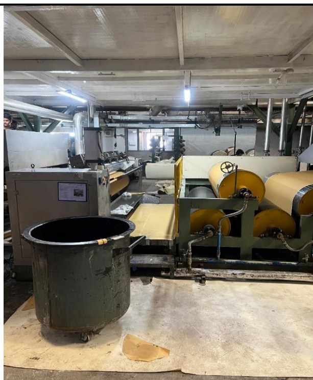
Machinery Name: Adhesive Head Location In Plant: Main Plant Use: Use water to cool down leather & paper temperatures
