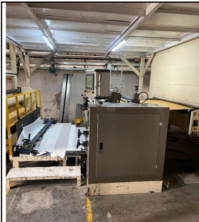
Machinery Name: Lacure Head Location In Plant: Main Plant Use: 1 st Coater With Printer
